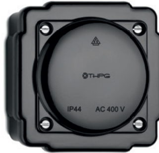
Junction box surface-mounted AC 400 V. For cables up to 4 x 2.5 mm 2 . 95 x 95 x 45 mm. Weight 140 g. IP44.
