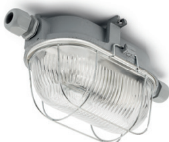
Oval cast iron basement lamp large Length 195 mm, width 135 mm, height 115 mm. Weight 1700 g. Porcelain socket E27, max. 100 W. IP54. Product code 100506
